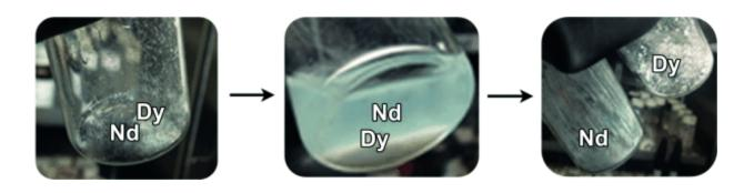
Rare-earth metals are critical components of electronic materials and permanent magnets. Recycling of consumer products is a promising source for these rare commodities. In the journal *Angewandte Chemie*, American scientists have now introduced a simple method for separating mixtures of neodymium and dysprosium salts—an important step towards recycling these valuable rare-earth metals.
