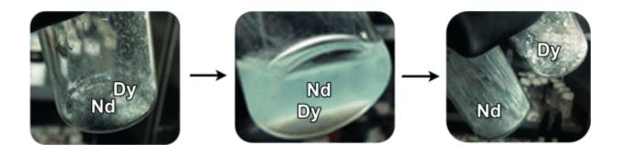
Rare-earth metals are critical components of electronic materials and permanent magnets. Recycling of consumer products is a promising source for these rare commodities. In the journal *Angewandte Chemie*, American scientists have now introduced a simple method for separating mixtures of neodymium and dysprosium salts—an important step towards recycling these valuable rare-earth metals.
