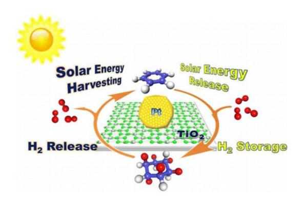
The new reversible hydrogen storage method stores hydrogen atoms in cyclohexane and uses solar energy to release the hydrogen atoms, turning the cyclohexane molecule into benzene. The use of solar energy avoids the need for high temperatures to release the hydrogen. Credit: Li, et al. ©2015 American Chemical Society
