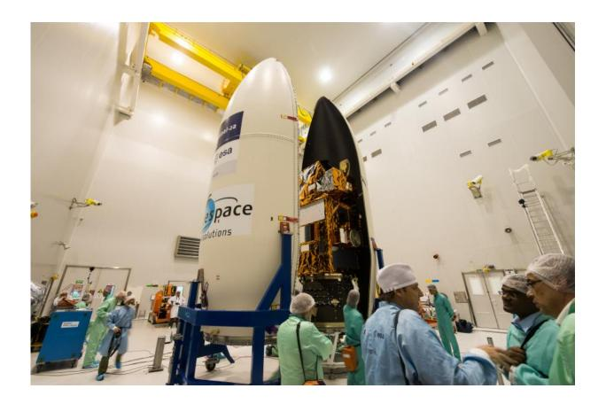
Sentinel-2A being encapsulated within the half-shells of the Vega rocket fairing. Credit: ESA–M. Pedoussaut, 2015
