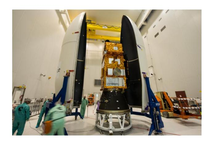
Sentinel-2A being encapsulated within the half-shells of the Vega rocket fairing. Liftoff from Europe's spaceport in Kourou, French Guiana, is set for 23 June at 01:52 GMT (03:52 CEST; 22:52 local time on 22 June), on 6 June 2015 at Europe's Spaceport in Kourou, French Guiana. Credit: ESA–M. Pedoussaut, 2015
