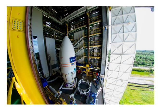
The Vega fairing holding the Sentinel-2A satellite in the launch gantry at Europe's Spaceport in Kourou, French Guiana. Credit: ESA–M. Pédoussaut
