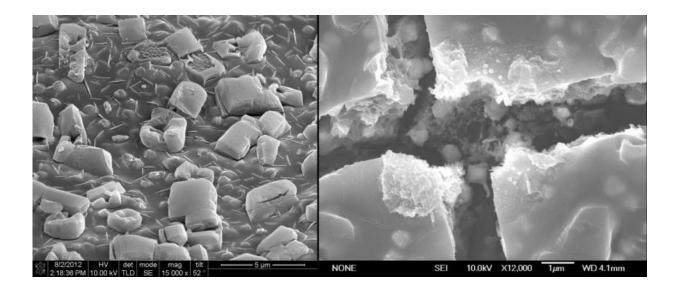
The phozographic paper before (left) and after (right) exposure seen through a scanning electron microscope. Credit: Jeff (Zhifeng) Huang/UCLA
