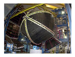
The CEBAF Large Acceptance Spectrometer, or CLAS, in Jefferson Lab's Experimental Hall B was used to measure electrons during the experiment.
