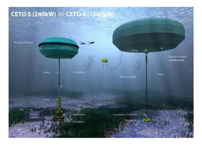
Artist' concept of a series of the Carnegie Wave Energy's tidal system, where buoys anchored to the sea floor and use swells to move a series of pumps. Credit: Carnegie Wave Energy
