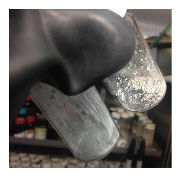
Because neodymium-ligand complexes bind together into dimers, their solubility is higher than the dysprosium-ligand monomers. This allows the former to be easily filtered off. Credit: University of Pennsylvania
