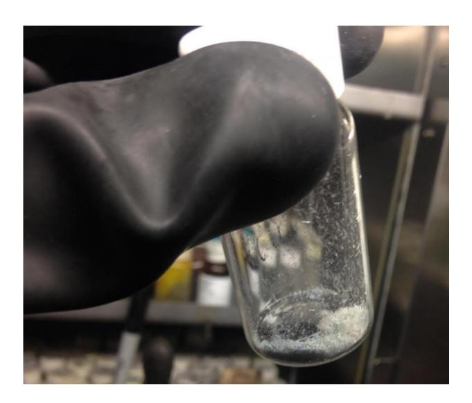
Starting with neodymium and dysprosium as a mixed powder, a metal-binding molecule known as a ligand is applied. Credit: University of Pennsylvania
