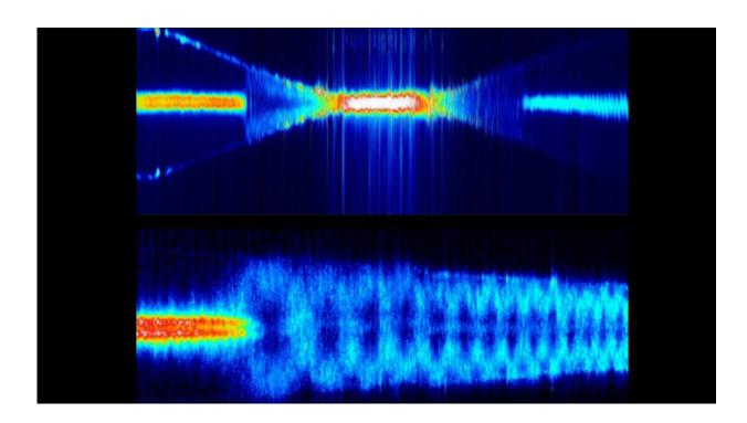
This technique directly images the propagation of light through an optical nanofiber, seen here as blue waves. The upper image is a zoomed out compilation of the Rayleigh scattering along the nanofiber. The saturated white section is the narrow neck of the nanofiber.
