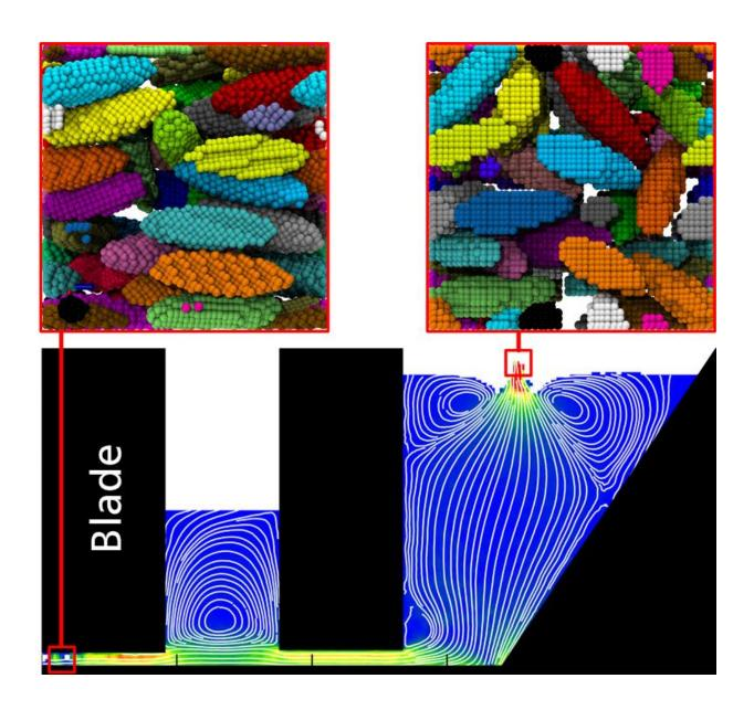
Bottom – macroscopic simulation: flow lines during the casting process. The
