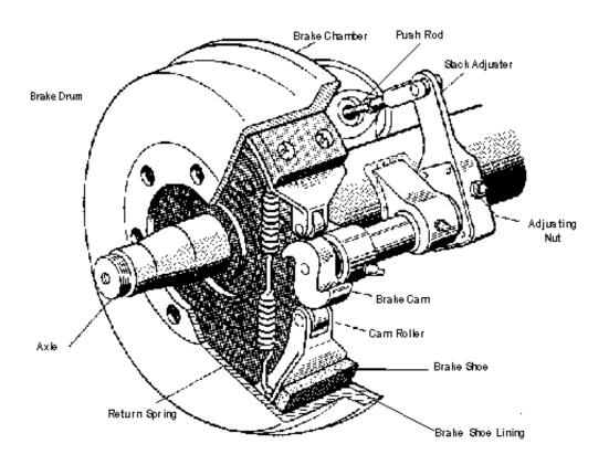
Even simple diagrams, such as this schematic of the working parts of a brake system, can help students construct a mental framework of how something
