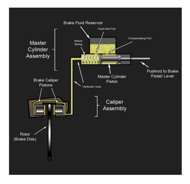
Animated diagrams with moving parts, such as this schematic of hydraulic braking systems, may be especially helpful to learning since they show both spatial relationship and real-time interaction of system components. Credit: WIKIPEDIA
