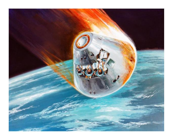
As spacecraft, like the Apollo Command Module depicted in this artist's concept, enter the atmosphere, a plasma sheath engulfs them that can cut off communication signals with the ground. Credit: NASA
