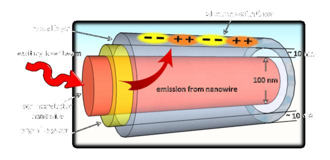
Simplified sketch of a plasmonic metal/organic/semiconductor nanowire heterostructure. The emission from the nanowire generated by the exciting laser beam is used as an energy pump to compensate for resistivity losses in the metal shell. An organic spacer layer of few 10 nm thickness is inserted to control this energy transfer. Credit: Hans-Peter Wagner and Masoud Kaveh-Baghbadorani, CC BY-NC-ND
