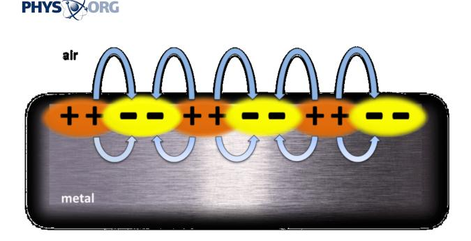
Simplified sketch of electron oscillations (plasmons) at the metal/air interface. Orange and yellow clouds indicate regions with lower and higher electron concentration, respectively. Arrows show electric field lines in and outside of the metal. Credit: Hans-Peter Wagner and Masoud Kaveh-Baghbadorani, CC BY-ND
