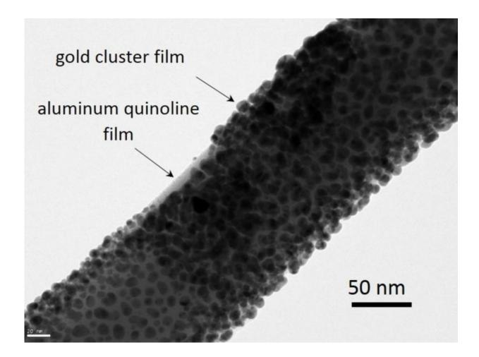
Transmission electron microscope (HRTEM) image of a GaAs-AlGaAs coreshell nanowire coated with nominally 10 nm aluminum quinoline and a 5 to 10 nm thick gold cluster film on top. Credit: Melodie Fickenscher (Advanced Materials Characterization Center College of Engineering and Applied Science)
