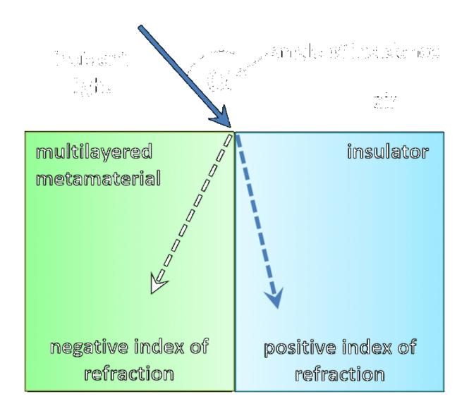
Light changes its direction when it enters a transparent insulator with positive refractive index or a metamaterial with negative refractive index. Credit: Hans-Peter Wagner and Masoud Kaveh-Baghbadorani, CC BY-ND
