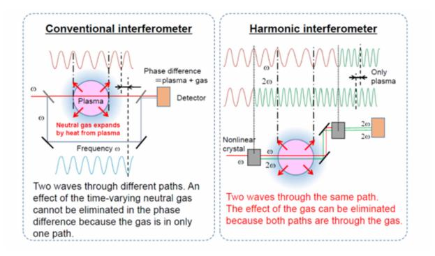
Reduction in influence of atmospheric pressure (gas) with harmonic interferometer. The interferometer can obtain information (density, etc.) of the medium from the time (phase) difference between two waves. Credit: NINS/NIFS
