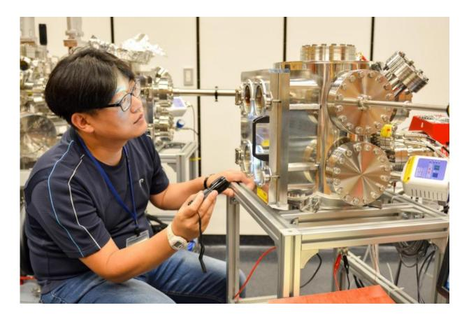
OIST staff scientist Min-Cherl Jung monitors the vacuum evaporation process in which spiro-OMeTAD powder is heated up inside and the molecules "snow" up, depositing a thin, even top layer onto the perovskite solar cell. Credit: OIST
