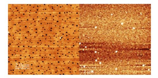
Atomic force microscopy (AFM) images show pinholes in the spiro-OMeTAD layer prepared by spin-coating (left) versus no pinholes when prepared by vacuum evaporation (right). Credit: OIST
