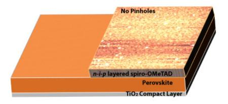
Many high-performance solar cells under development layer spiro-OMeTAD on top of perovskite, with other trace elements added to increase electrical conductivity. Credit: OIST
