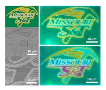
Missouri S&T researchers have developed a method to accurately print high-resolution images on nanoscale materials. They used the Missouri S&T athletic logo to demonstrate the process. At top left is the original logo. At right are examples of the logo printed at the nanoscale level.
