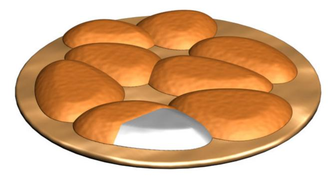
These illustrations show deposits that form on the cathode of a lithium metal battery. When lithium nitrate is added to the electrolyte, destructive 'fingers' of lithium metal, known as dendrites, grow on the surface. When lithium polysulfide is added as well (orange image), harmless pancake-like deposits form instead. Credit: W. Li et al, *Nature Communications*
