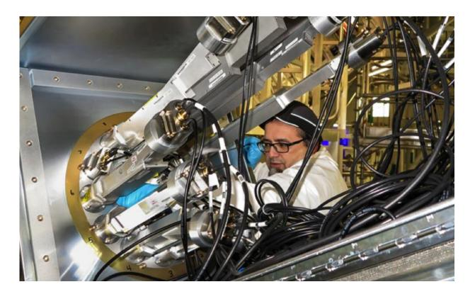
Target area operator Sky Marshall installs new apertures in the Dante 2 X-ray diodes. Credit: James Pryatel/LLNL
