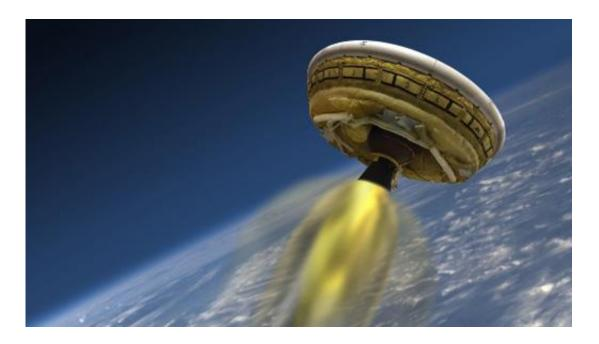
This NASA artist's concept obtained June 2, 2015 shows the test vehicle for NASA's Low-Density Supersonic Decelerator, designed to test landing technologies for future Mars missions
