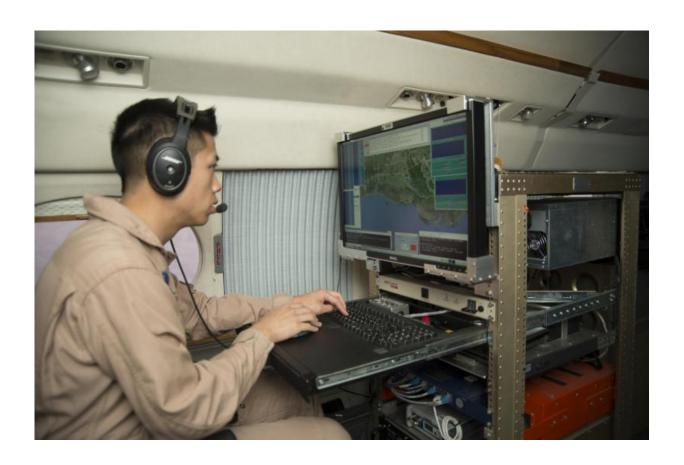
Kean Tam, UAVSAR instrument operator, monitors the C-20A's flight path to ensure that accurate data are collected. Credit: NASA
