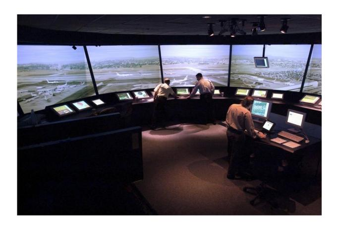
NASA Future Flight Central is a national Air Traffic Control/Air Traffic Management (ATC/ATM) simulation facility. The two-story facility offers a 360-degree full-scale, real-time simulation of an airport, where controllers, pilots and airport personnel participate to optimize expansion plans, operating procedures, and evaluate new technologies. Credit: NASA
