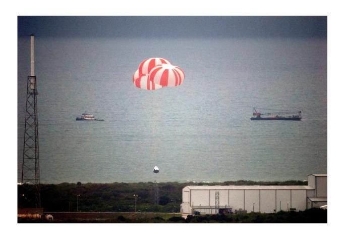
SpaceX's Crew Dragon spacecraft splashed down in the Atlantic Ocean under three main parachutes following a successful test on May 6, 2015 of the spacecraft's ability to save astronauts in the unlikely event of a life-threatening situation on the launch pad. Credit: NASA
