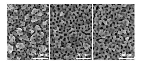
Electron micrographs of nanoporous gold materials that were fabricated using different sizes of micelles. Pore size increases from left to right.
