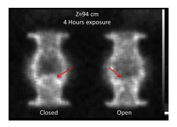
Muon tomography images of a valve allowed researchers to differentiate between an open and closed valve. Credit: Matt Durham, Los Alamos National Laboratory
