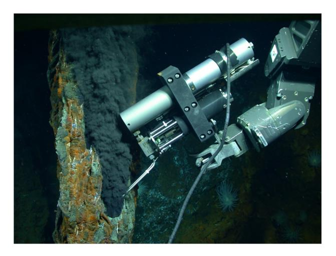
Vent fluid samples were collected using titanium isobaric gas-tight (IGT) samplers deployed by the remotely operated vehicle Jason aboard the R/V Atlantis in January 2012. The IGTs, unique instruments developed by Jeff Seewald and a team of WHOI engineers, are designed to maintain the sample fluid at the high pressure at which it was drawn. Credit: Chris German, WHOI/NASA, NSF/ROV Jason/Woods Hole Oceanographic Institution
