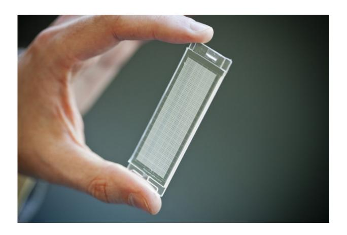
Love holds a microfluidic device, developed in Hidde Ploegh's lab, that resembles a tiny ice cube tray, with individual compartments for each cell. Love and Ploegh designed the device, which can be used to isolate many individual cells and simultaneously measure the antibodies and other proteins that each cell secreted. Credit: Dominick Reuter
