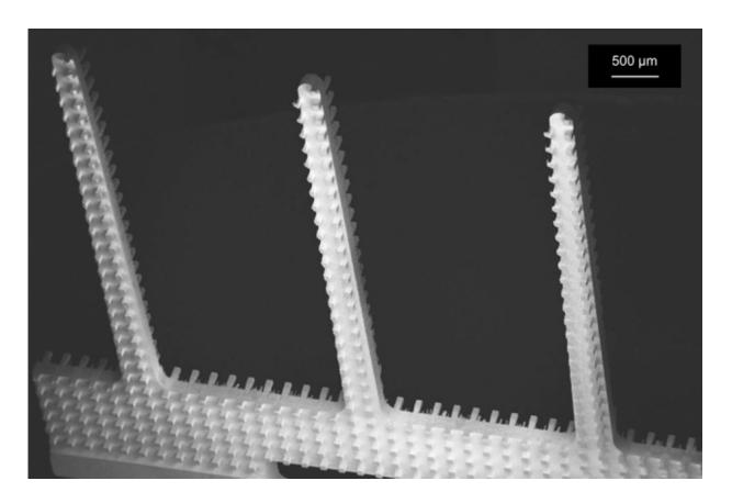
A scanning electron micrograph of the new microfiber emitters, showing the arrays of rectangular columns etched into their sides.
