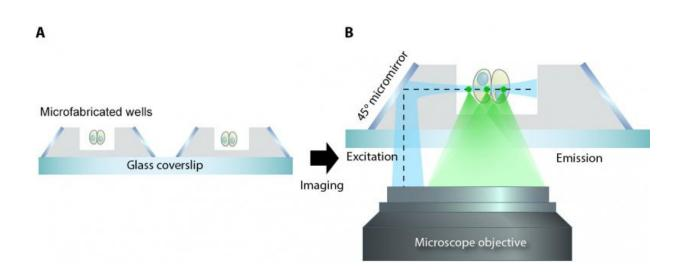
Figure: Schematic showing the soSPIM technique. A) Cells can be grown in the microfabricated wells, holding them in place for imaging. B) The 45° micromirrors reflect the excitation beam (dotted line) from a single objective, through the sample, and the resultant emitted fluorescence signal is captured by the same objective.
