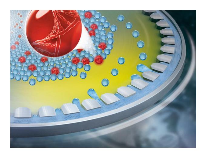
3D illustration of droplet formation on a lab-on-a-chip system: Drops of water tear off from the mouths of the channels as the disk rotates. A layer of oil ensures that the drops do not combine again. Credit: Hahn-Schickard
