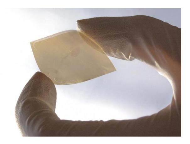
A photograph of a single-flake-layer WSe2 thin film deposited on flexible Sn:In2O3 (ITO)-coated PET plastic. Credit: Kevin Sivula/EPFL
