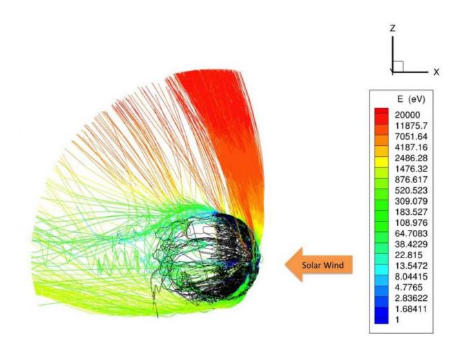
Computer simulation of the interaction of the solar wind with electrically charged particles (ions) in Mars' upper atmosphere. The lines represent the paths of individual ions and the colors represent their energy, and show that the polar plume (red) contains the most-energetic ions. Credit: X. Fang, University of Colorado, and the MAVEN science team
