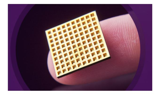
A version of Microchip Biotech's implantable, wirelessly controlled microchip. When an electrical current is delivered to one of the chip's tiny reservoirs, a single dose of therapeutics is released into the body. Credit: Microchips Biotech
