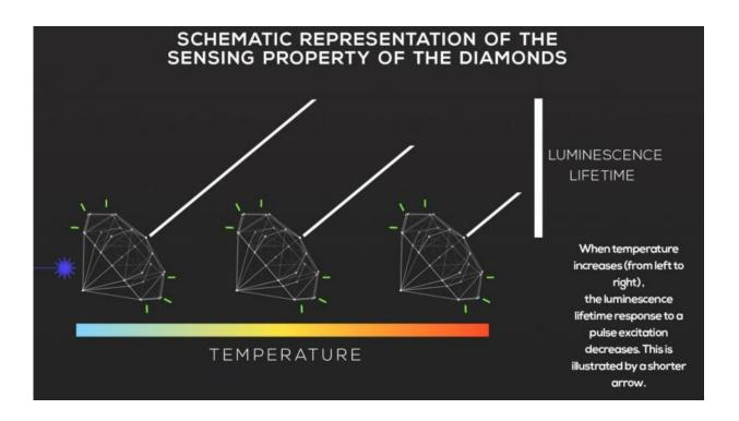
A schematic representation of the temperature sensing properties of diamond defects. Credit: Homeyer, et al./ Université de Lyon
