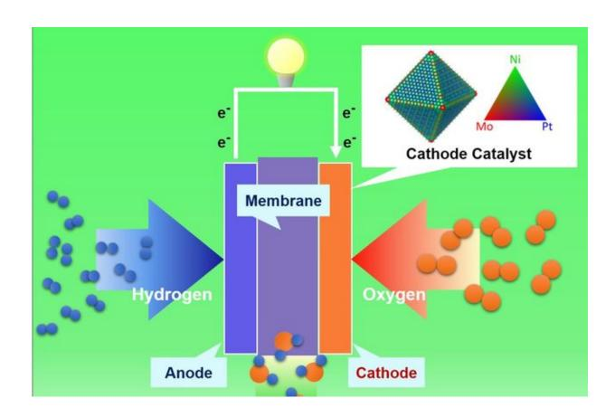
Diagram of a proton exchange membrane fuel cell created using a surface engineering technique called "surface doping." Credit: Yu Huang Lab/UCLA
