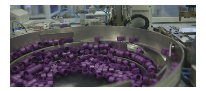
Gas sensors being made. Credit: credit Alphasense
