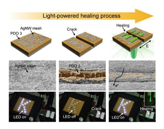
Light-powered healing of electrical conductor: (left to right) pristine, cracked, and optically-healed electrical conductor. Credit: KAIST
