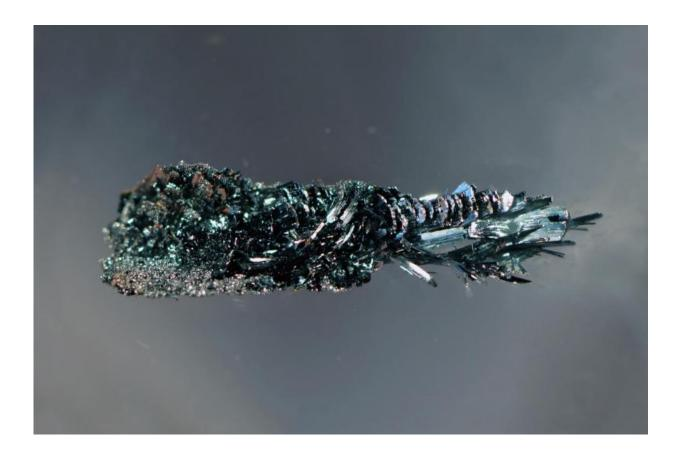
Crystals of black arsenic phosphorus -- exchanging phyphorus against arsenic, the band gap can be tuned to as low as 0.15 eV, making the material predestined for long wavelength infrared sensors. Credit: Andreas Battenberg / TUM
