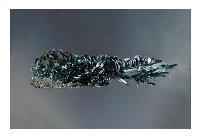
Crystals of black arsenic phosphorus -- exchanging phsphorus against arsenic, the band gap can be tuned to as low as 0.15 eV, making the material predestined for long wavelength infrared sensors. Credit: Andreas Battenberg / TUM
