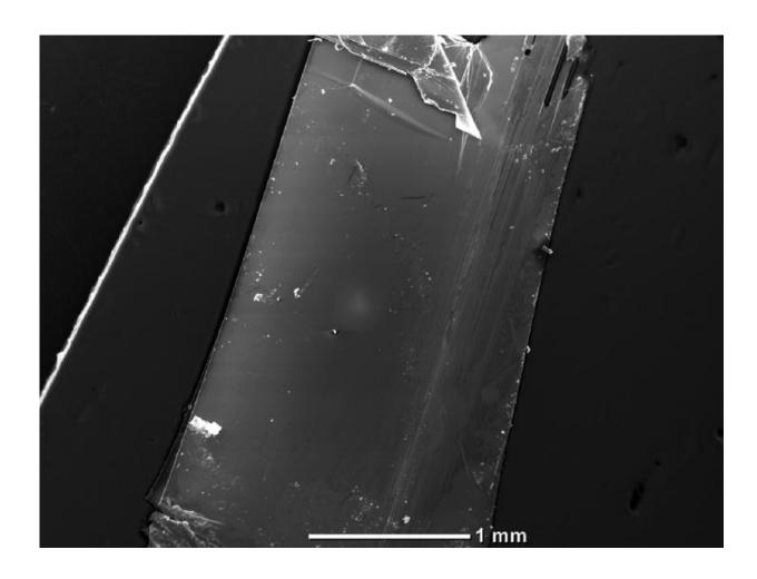
Electronmicroscopic image of a single crystal of black arsenic phosphorus. At the upper rim beginning delamination is visible. By careful delamination films as thin as two atomic layers were obtained. Credit: Marianne Koepf / TUM
