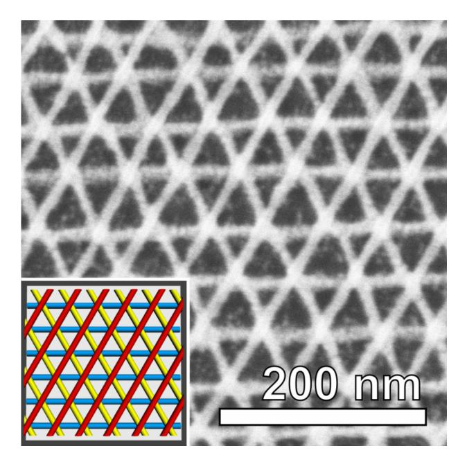
Scanning electron microscope image of a three-layer platinum mesh. The colored inset shows each distinct layer of the nanoscale grid. Credit: Brookhaven National Laboratory
