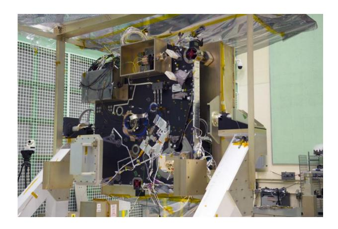
The lasers and optics of the ATLAS instrument are fixed into place on a flat bench structure, seen here in March 2015 before it was attached to the instrument's box structure and connected to the electronics. Credit: Debora
