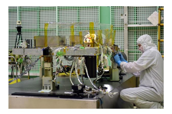
The optical bench on ICESat-2's instrument, called the Advanced Topographic Laser Altimeter System (ATLAS), holds most of the components needed to direct the laser from its source on the instrument – the gold colored boxes seen here – to Earth's surface. Credit: Ryan Fitzgibbons, NASA Goddard
