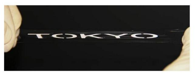
An elastic conductor was created by a one-step printing process on a sportswear material. The top shows the elastic conductor at its original length. The middle and bottom images show the stretched elastic conductor at about two times and over three times its original length. The elastic conductor exhibited high conductivity even when it was stretched to more than three times its original
