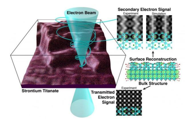
A highly promising technique called "high-resolution scanning electron microscopy," or HRSEM, extends scanning microscopy to the atomic scale and provides information on both surface and bulk atoms simultaneously.
