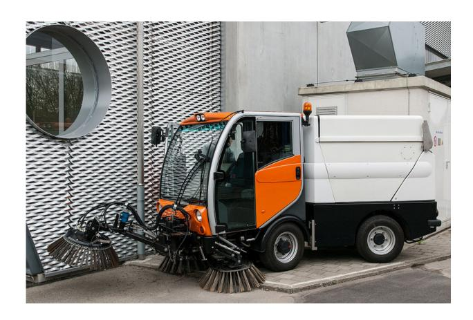
Empa, ETH Zürich and the road sweeper manufacturer Bucher Municipal have jointly developed a pioneering hybrid-electric powertrain for road sweepers in a CTI project. The concept is based on a
