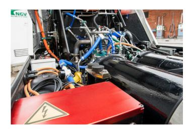
The hybrid drive system has a modular design. This means that a petrol, liquefied petroleum gas or diesel engine could be installed instead of a natural gas engine. If a hydrogen-powered fuel cell or a significantly larger battery is used instead of an internal combustion engine with power generator, purely electrical operation would also be possible. This modular drive concept will allow Bucher Municipal to cater for a wide range of different customer needs in the future.
