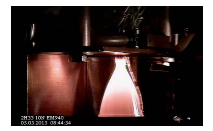
The world's first spacecraft thruster with a platinum combustion chamber and nozzle made by 3D printing has passed its baptism of fire with a series of firings lasting more than an hour and 618 ignitions. The firings included a single burn of 32 minutes, during which a maximum throat temperature of 1253°C was attained. Credit: Airbus Defence & Space
