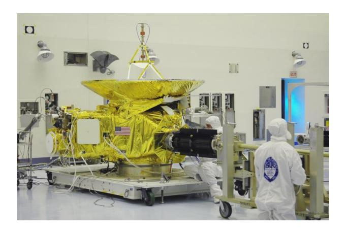
Engineers perform a test fit of New Horizons' RTG. Credit: NASA/KSC
