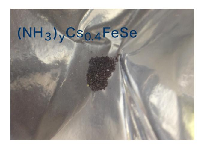
Figure 1. The  $(NH_3)_v Cs_{0.4}$ FeSe sample prepared by liquid ammonia technique.
