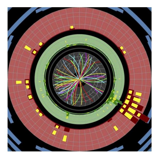
Protons collide at 13 TeV, sending showers of particles through the ATLAS detector during tests on May 20. Credit: ATLAS
