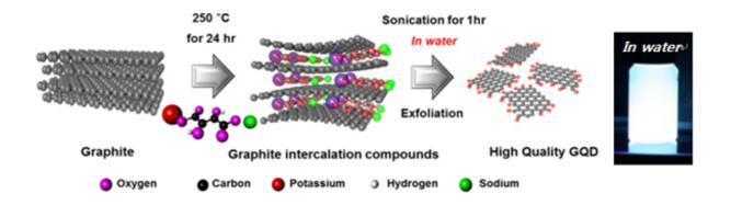
A schematic illustration of the preparation method of highly efficient GQDs (left) and an image of GQDs dispersed in water (right). Credit: KAIST
