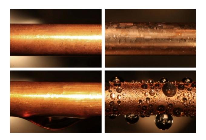
An uncoated copper condenser tube (top left) is shown next to a similar tube coated with graphene (top right). When exposed to water vapor at 100 degrees Celsius, the uncoated tube produces an inefficient water film (bottom left), while the coated shows the more desirable dropwise condensation (bottom right).
