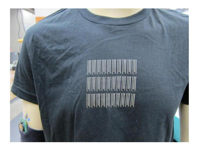
Garment-based printable electrodes developed in the lab of Joseph Wang, distinguished professor of nanoengineering at UC San Diego, and lead principal investigator of ATTACH. Credit: Jacobs School of Engineering/UC San Diego
