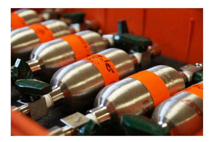
The cylinders Jim Boles used to gather casing gas samples from oil wells along the Newport-Inglewood fault, where he found evidence of helium-3. Credit: Sonia Fernandez
