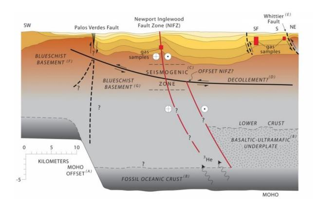
A geologic cross section of the Los Angeles Basin from the southwest to northeast. This profile intersects the Newport-Inglewood Fault Zone at Long Beach.
